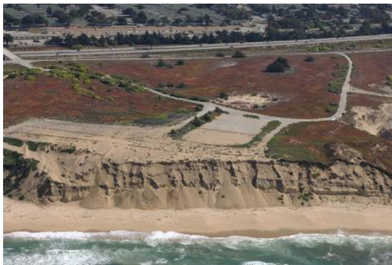
Figure 6-2. The Former Officers Club at Stillwell Hall on Ford Ord. (A) Revetment reduced erosion but resulted in the loss of the beach (2002). (B). Following removal of the revetment and equilibrating erosion, the beach returned as the dune eroded (2005). Photos courtesy of the California Coastal Records Project
